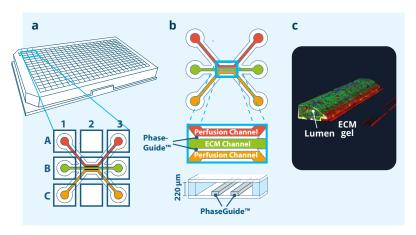
(a) The OrganoPlate® 3-lane 40 lay out and chip design. The plate contains 40 microfluidic chips with 3 channels. (b) The 3 channels are adjacent in the observation window. The PhaseGuides tm allow for use of extra cellular matrix (ECM)-like gel in the middle channel. There are no artificial membranes between the ECM channel and perfusion channels. (c) 3D IHS staining of intestinal (Caco-2) tubules cultured in the OrganoPlate 3-lane 40.
