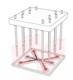
The electrode board of the OrganoTEER® is lowered into the wells of the OrganoPlate®
