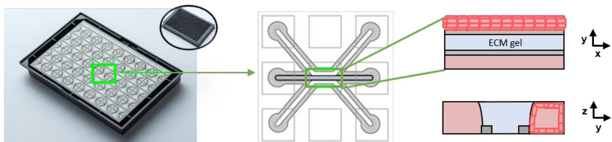
**Figure 1: Endothelial tubules in the OrganoPlate® 3-lane.** The OrganoPlate® 3-lane holds 40 microfluidic chips that can be used to culture miniaturized tissue- and organ models. Each chip holds three channels. The middle channel is used to seed an extracellular matrix (ECM) gel and the top channel can be used to grow an endothelial vessel. The bottom channel can be used to supply cells with medium or to add compounds, such as an angiogenic cocktail.
