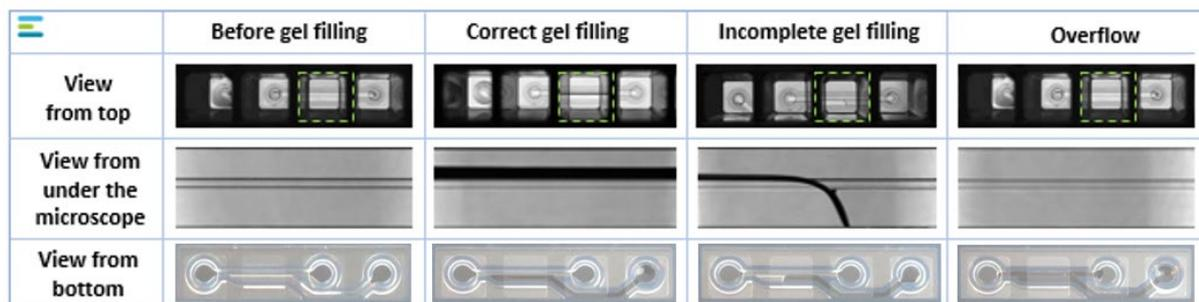
**Figure 5:** Overview of correct gel filling, incomplete gel filling, and overflow in the OrganoPlate® 2-lane. Note: images show filling of gel without cells and function only as an example to demonstrate correct gel seeding.
