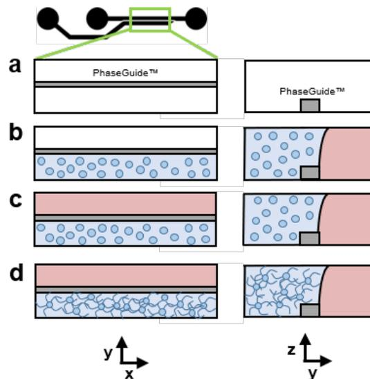
*Figure 3: Schematic representation of CNS cell seeding in ECM gel in the OrganoPlate® 2-lane*
