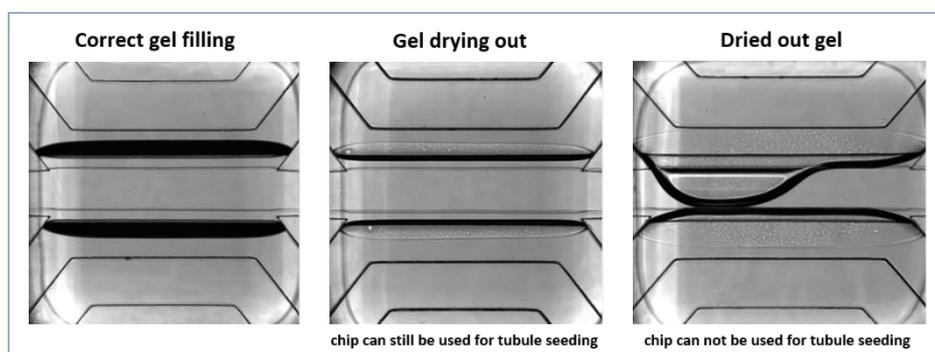
**Figure 9:** ECM gel drying out due to prolonged gel loading or polymerization
