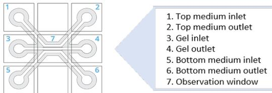
**Figure 1:** Schematic representation of an OrganoPlate® 3-lane tissue chip.
